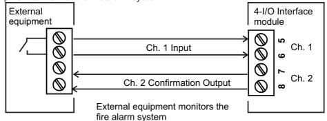
The confirmation output will operate within 1s of the input being accepted (design must also allow for any input delay settings).
