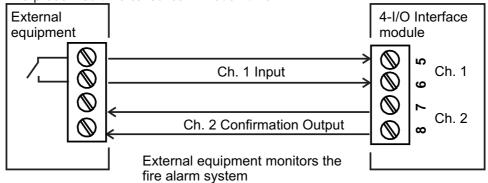
The acceptance of an active input signal can be delayed until it has remained active for a set period of time. Additionally a verbose / silent (non verbose) setting is available. The verbose setting allows supervisory message indication on change of input state and a timeout fault, given if a change of state has not occurred within the confirmation time duration. The silent setting will only give a timeout fault. This facility allows the fire alarm system to monitor external equipment.
