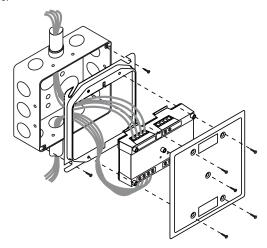
SIGA-MCC1 and SIGA-MCC2: mount the UIO motherboard inside a suitable GE Security enclosure with screws and washers provided. Plug the SIGA-MCC1 or SIGA-MCC2 into any available position on the motherboard and secure the module to the motherboard with the captive screws. Wiring connections are made to the terminals on the motherboard (see wiring diagram). UIO motherboard terminals are suited for #12 to #18 AWG (2.5 mm² to 0.75 mm²) wire size.
